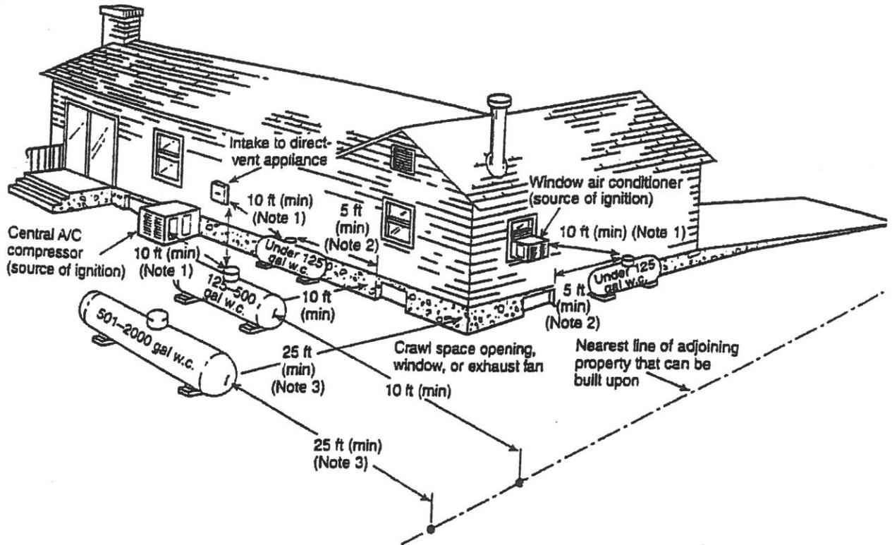
Regardless of its size, any ASME container filled on site must be located so that the filling connection and fixed maximum liquid level gauge are at least 10 ft from any external source of ignition (e.g., open flame, window A/C, compressor), intake to direct-vented gas appliance, or intake to a mechanical ventilation system.
